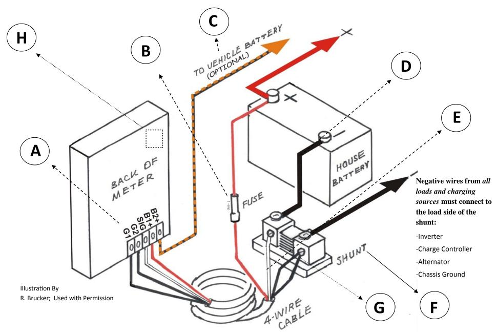
**REQUIRED:** 4-Wire Cable and Electrical Shunt
